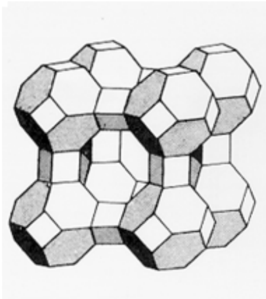
Fig 1. Zeolite (Clinoptilolite) crystal structure.
